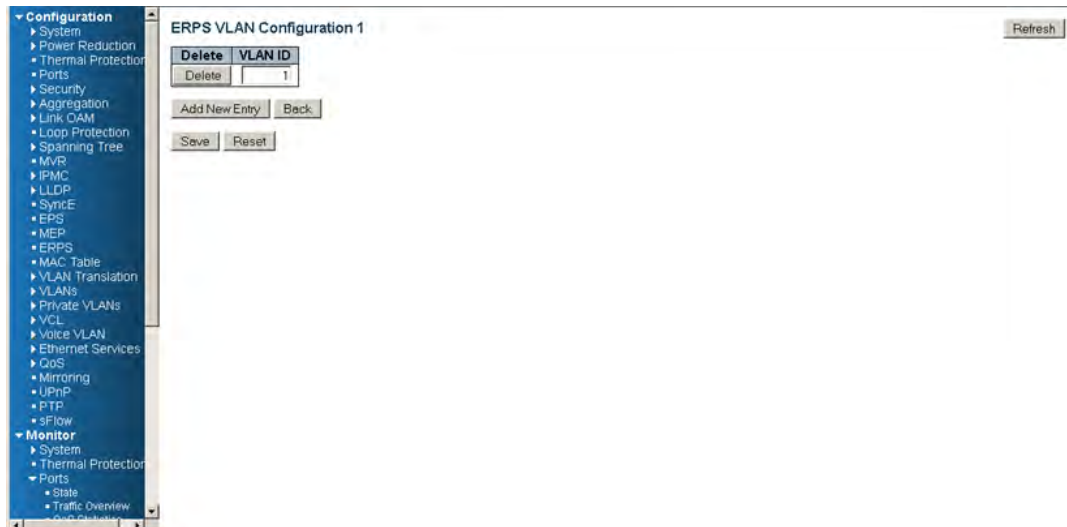
Figure 20 • Protected VLAN (Switch 2) Configuration
