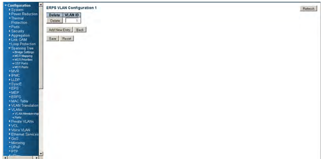
Figure 16 • Protected VLAN (Switch 1) Configuration
